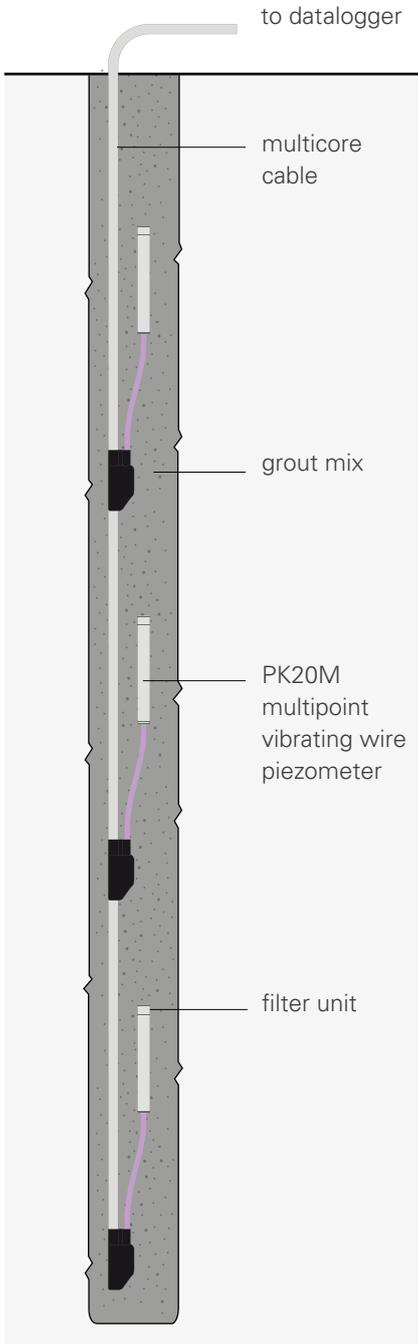
The fully-grouted installation method provides a reliable way to install piezometers in the same borehole, each measuring pore-water pressure at a different elevation. It eliminates problems with placing sand intake zones, bentonite seals, and channeling of water along signal cables.
